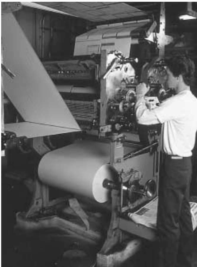
Web presses are used to manufacture newspapers, magazines, and books.
